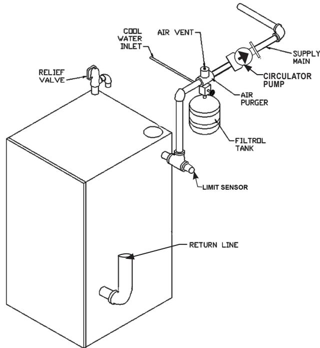
Figure 5 - Chilled Water Piping
