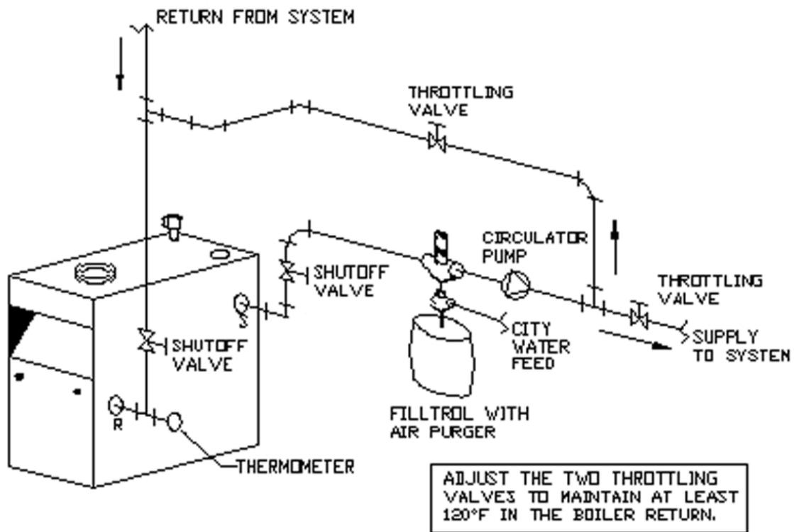
Figure 7 - BYPASS PIPING - CIRCULATOR ON RETURN
