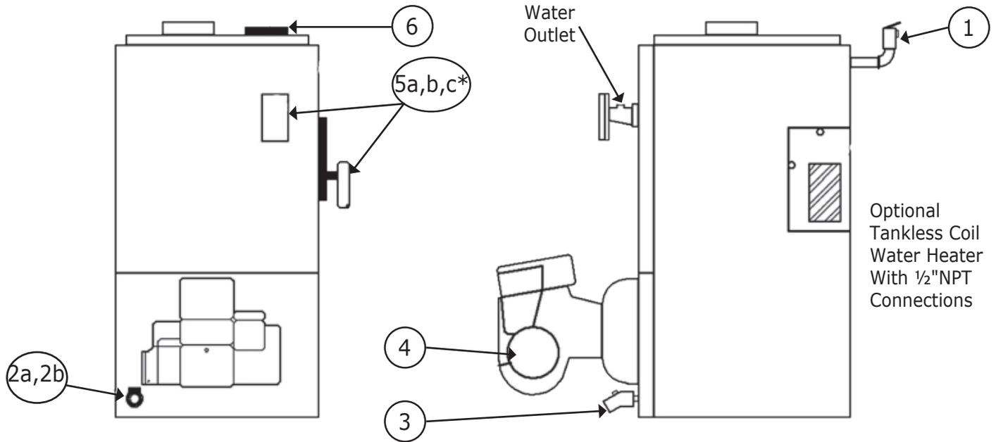
\* Item 5a Hydrolevel limit control is located on front supply tapping for less-coil boilers and on tankless coil cover plate for with-coil boilers. Note different control well used in each location.
